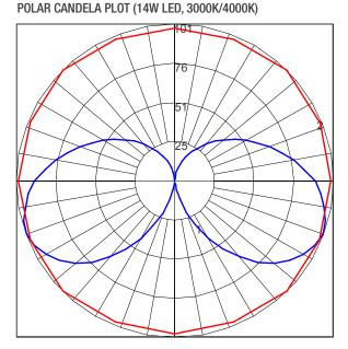
Maximum Candela = 101.12 Located at Horizontal Angle = 45, Vertical Angle = 70 #1 - Vertical Plane Through Horizonal Angles (45 - 225) (Through Max. Cd.) #2 - Horizontal Cone Through Vertical Angle (70) (Through Max. Cd.) ISOFOOTCANDLE PLOT (14W LED, 3000K/4000K)
