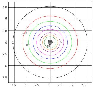
Isofootcandle Plot shows light distribution pattern at ground level with LED light board. Readings have been taken assuming the photometric center of the luminaire to be 0.51 feet above ground level. IES files for standard lamps are available on our website.
